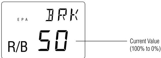
**Note:** If Grip Lever A is assigned an Auxiliary Channel 3 function by selecting “LN” or “2P” with Grip Button C in use, the Brake End-Point Adjustment will not be available.
