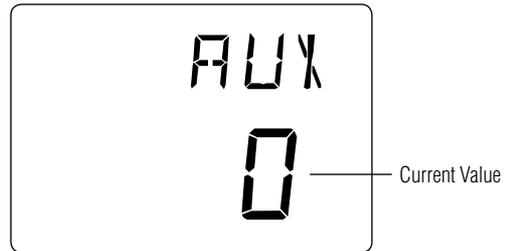
When the LN (linear) Auxiliary Channel 3 function is selected, Grip Lever A can be used to change the neutral position of the servo to lean or richen the engine’s fuel mixture. Once the desired fuel mixture has been achieved, the Grip Lever A value indicated on this screen can be transferred manually to the Sub-Trim function and the value of the AUX screen can be returned to zero. Please refer to diagram A below for proper grip lever operation.
