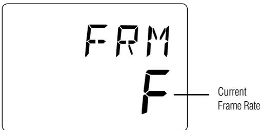
**Note:** The Frame Rate function offers quicker response times in the “F” or Fast mode. Some models of analog servos are not compatible in the “F” Fast mode and require the radio to be operated in the “N” Normal mode.
