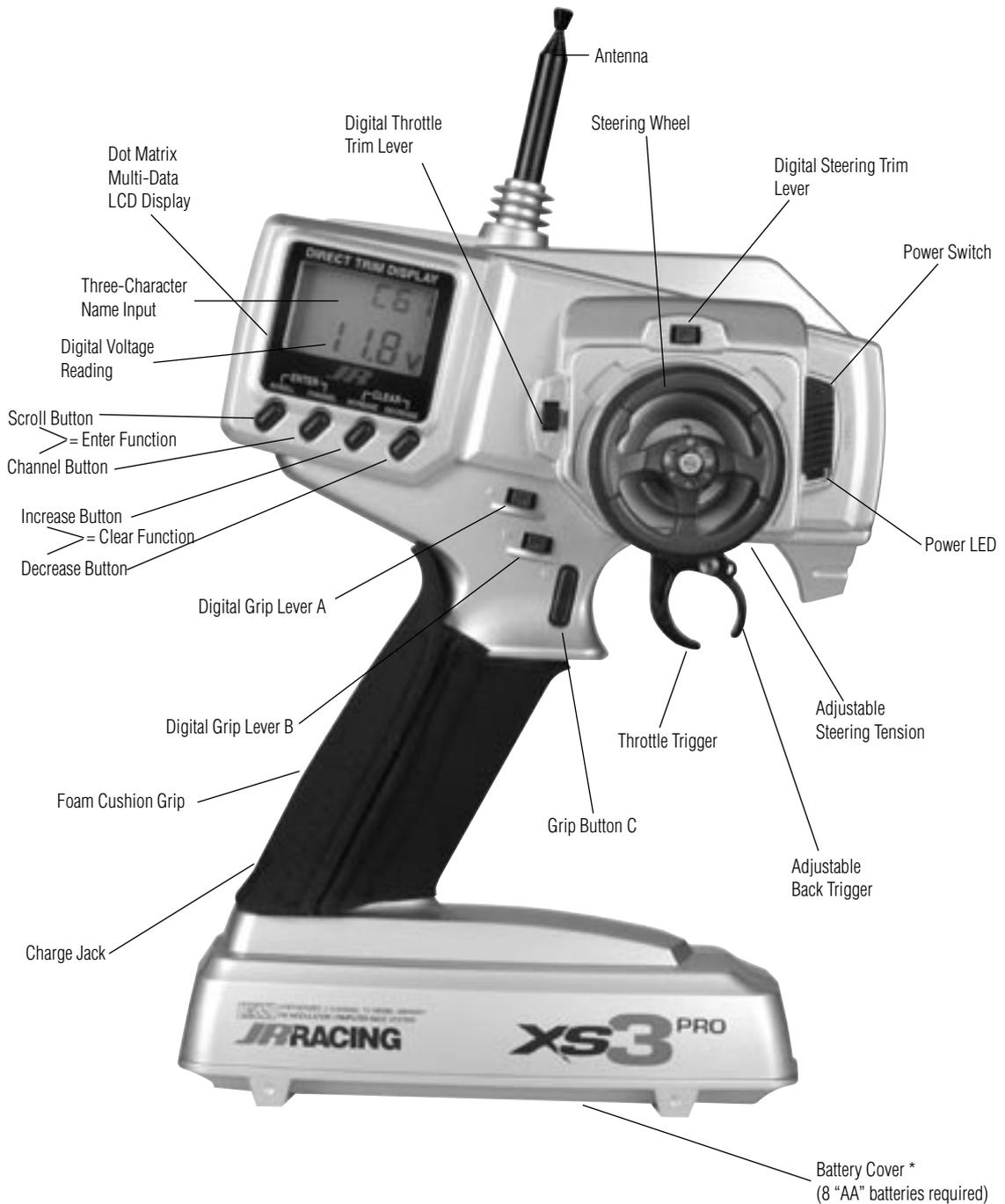
\*To remove battery cover, press down on the arrow and push the cover in the direction of the arrow. Remove the battery case and install 8 "AA" batteries in the direction shown as molded into the battery case. If transmitter voltage fails to register, check for correct battery installation and voltage.
