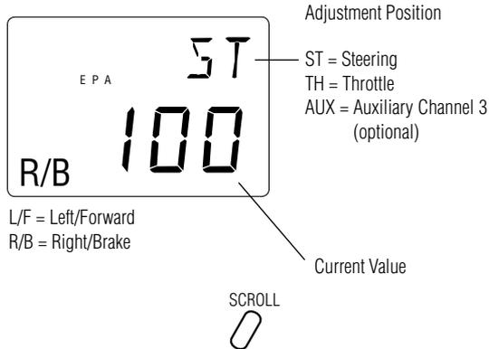
1. From the Servo Reverse function, press the *Scroll* key four times to access the End-Point (Travel) Adjustment function (the EPA screen with "ST" will appear).
