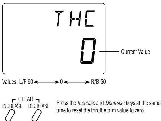
Each click will provide  $0.3^\circ$  of trim to the throttle servo with a maximum of  $24^\circ$  allowed.
