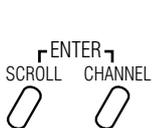
Press and hold the *Scroll* and *Channel* keys at the same time while turning the transmitter power switch on. Next, press the *Scroll* key until "CLR" appears.
