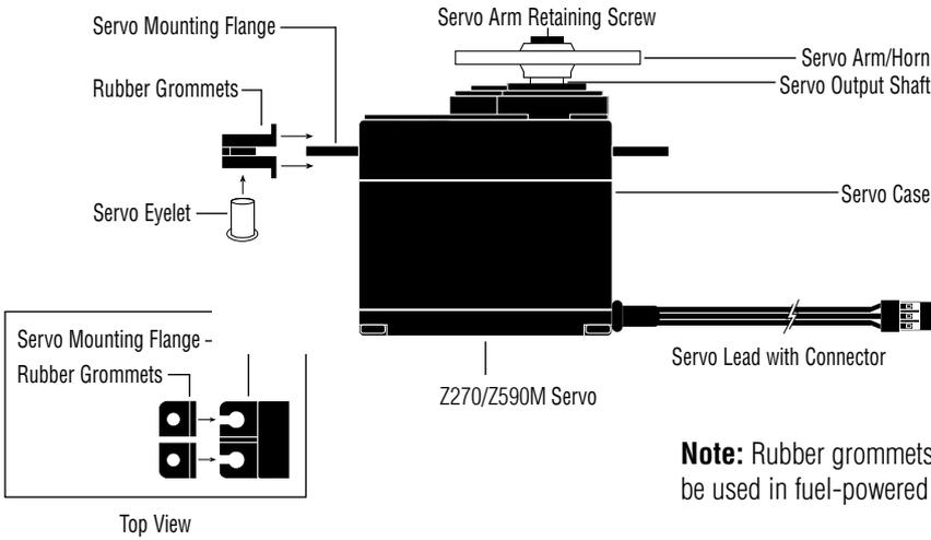
**Note:** Rubber grommets and eyelets must be used in fuel-powered vehicles.
